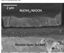
Fig. 1 Example 1: Ni(OH)2/NiOOH deposited on a passive layer (e.g. Ni) by anodic electrodeposition
