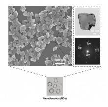
The new method requires an additional step, namely mixing the NDs with a specific amount of salt crystals such as sodium chloride prior to carrying out conventional oxidation. The use of SAAO results in ultra-clean NDs that emerge from the cleaning process visibly whiter in colour compared to the grey-tinged outcome that results without the use of SAAO. The new method will allow the cleaning of NDs to be scaled-up to enable them to be manufactured in large quantities and at low cost.
